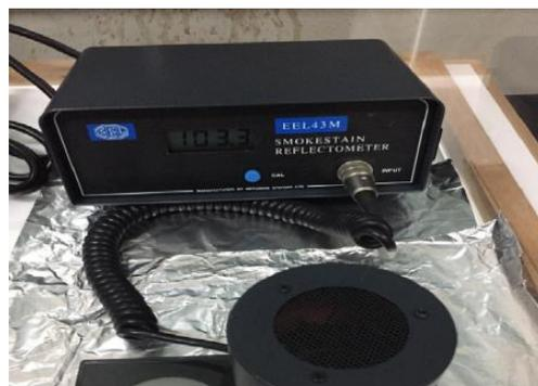
Fig. 4: EEL43M Smoke Stain Reflectometer (SSR)
